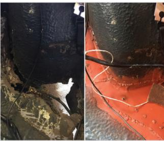
helped him prepare the 2000 ready for the new metal whilst I was at work. By the end of the bank holiday the new metal work was neatly fabricated and welded into place. Grateful to Nigel for his assistance, the 2000 was delivered straight to the MOT garage which she passed with an advisory on the 58
