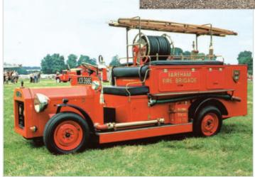
sonnel of Fareham Fire Station on a refurbished Triumph Herald chassis. Carries a crew of four, is equipped with a Hathaway/BSA 420 cc pump and 35 gallon water tank; one hose reel, 4-35 ft lengths of 1 ¾ in hose, and a No. 0 foam making branch. Carries a short trussed Ajax extension ladder. Used
