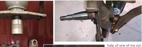
chining differences over the last 40 years separated them, they were to all intents and purpose identical where it mattered. New spindle inserted I used an air gun to 'hammer' home the new nut and pull the taper firmly home. This was then torqued to 65Nm.
