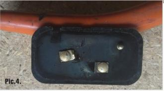
copper rivets that hold the external spade connectors in place (photo 4).
