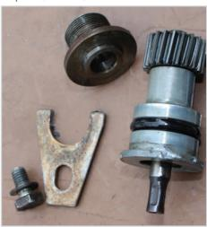
gear (NKC48). Pic.2. J-type speedo driven gear Assy. Doing the sum
