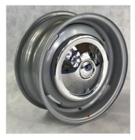
Pic.5. Weller wheel with Triumph hubcap
